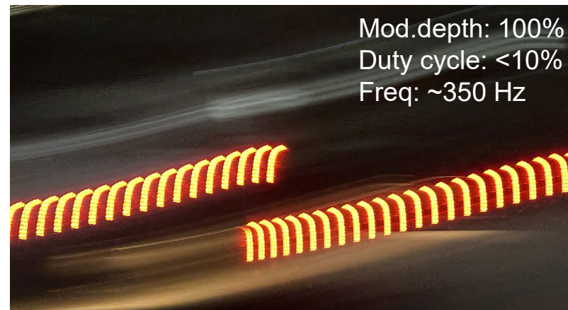
Figure. Illustration of the phantom array effect using a mobile camera, steady (top) and rapidly rotated (bottom).
