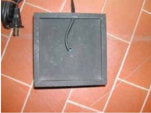
Missing cord anchorage for supply cable
