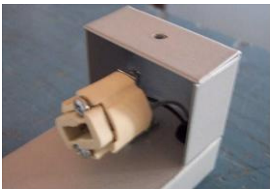
Wires with single insulation shall not touch metallic parts not earthed, and shall not be accessible
