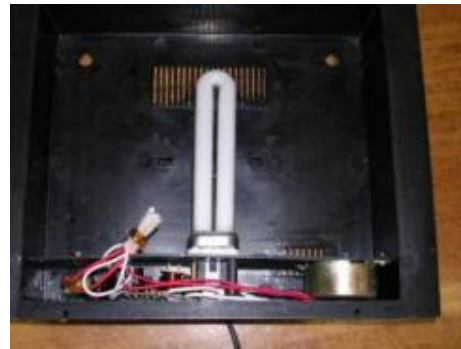
Accessible live parts during lamp replacement
