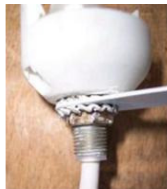
The lampholder doesn't twist under a 2 Nm torque test
