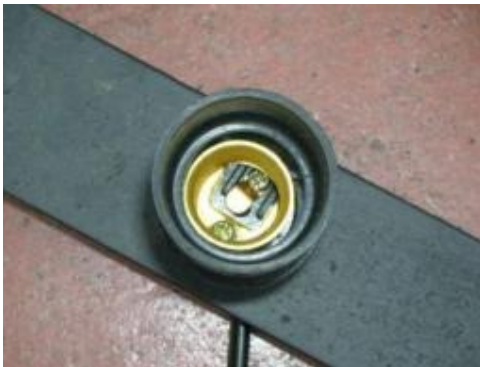
Live screw shell in the lampholder
