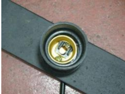
Live screw shell in the lampholder
