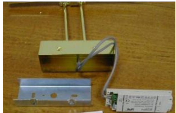
Example of metal part not connected to earth
